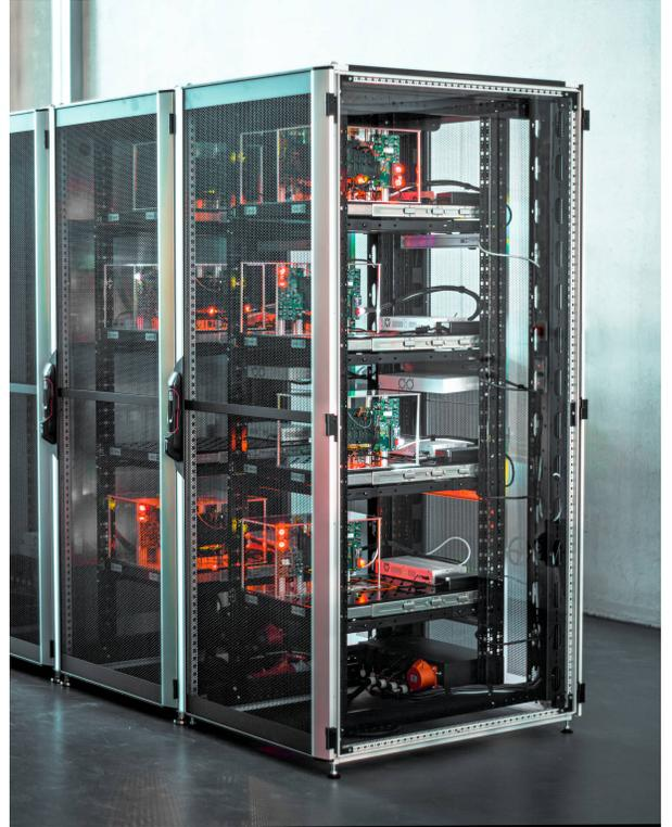
Figure 1. BrainScaleS-2 platform in the machine hall of the European Institute for Neuromorphic Computing. Two rack cabinets house up to 16 systems, each containing two ASICs. They are placed on retractable drawers to allow convenient access for maintenance. Each of these contains all components for operation, requiring only mains supply and a single Ethernet uplink. Both are supplied using local cable passages through the floor to the server room beneath (not visible in the picture).
