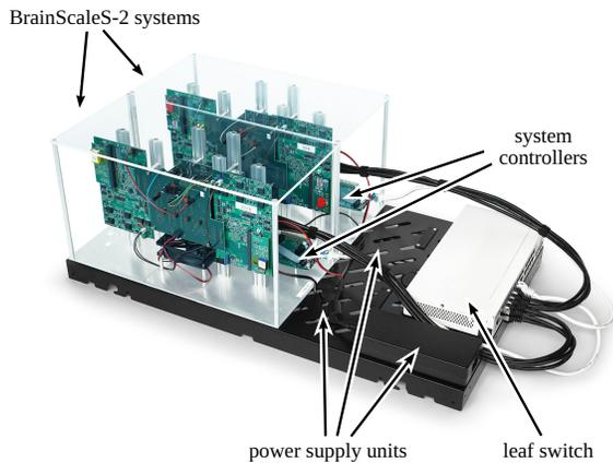
Figure 3. A single drawer of the BrainScaleS-2 platform, containing two systems<sup>2</sup> and all necessary periphery for operation from mains power and a single 10 GbE uplink. This includes ARM-based system controllers, three power supply units and the leaf switch also shown in Fig. 2.
